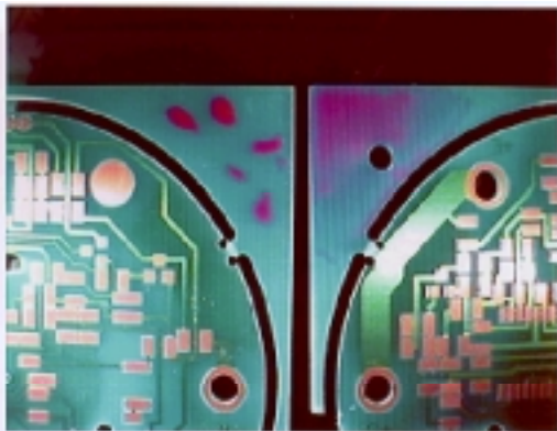
FIGURE 4 - Before/After Plasma Treatment on FR4
