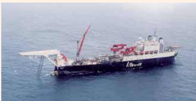
Allseas' dynamically positioned pipelay vessel Solitaire
